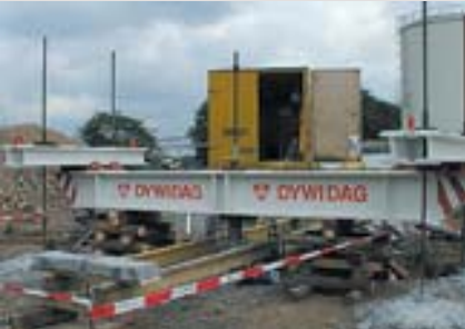
i Project Budenheim near Mainz, Germany DSI Services Performance test for grouted test piles Ø 118 x 9 mm
