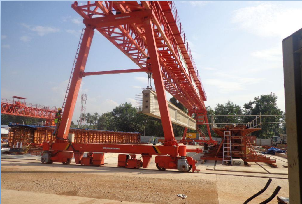
45m span 100 ton gantry crane
