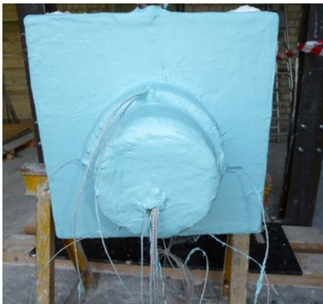
Coating before Fire Testing
